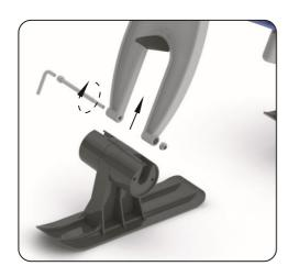
Slide the front ski assembly between the let of the fork. Tighten the front axle nut and bolt securely using the 6 mm hexagon allen wrench (I).
