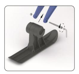
5 Slide the rear ski assembly between the legs of the frame. Tighten the rear axle nut and bolt securely using the 6 mm hexagon allen wrench.
