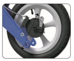
When the frame is separated from the rear-wheel assembly, allow the frame to drop downward. Remove the brake cable from the drum and use the supplied zip tie (part H) to secure the end to the frame.
